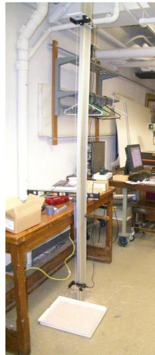
*Photogate set-up: Note the separation of the gates and the plumb-bob to assure that the balls pass through the center of both gates. The tray at the bottom is replaced with bubble wrap or cloth in your version of the experiment.*
