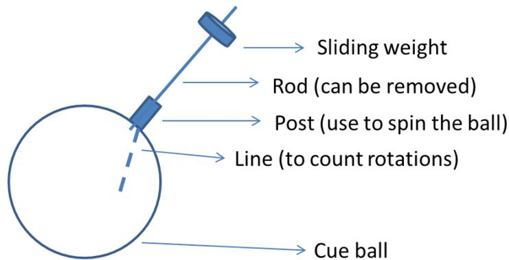
*The gyroscope. Note that the rod with the sliding weight can be removed. The line (which you should draw on the ball if it is not already there) is used in conjunction with the video camera to determine the rotation frequency of the ball.*
