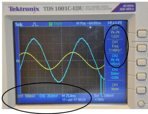
Use the CH1 Pk-Pk and CH2 Pk-Pk readings. Ignore the others. The frequency measurement here is not particularly accurate. Use the reading on the function generator instead.
