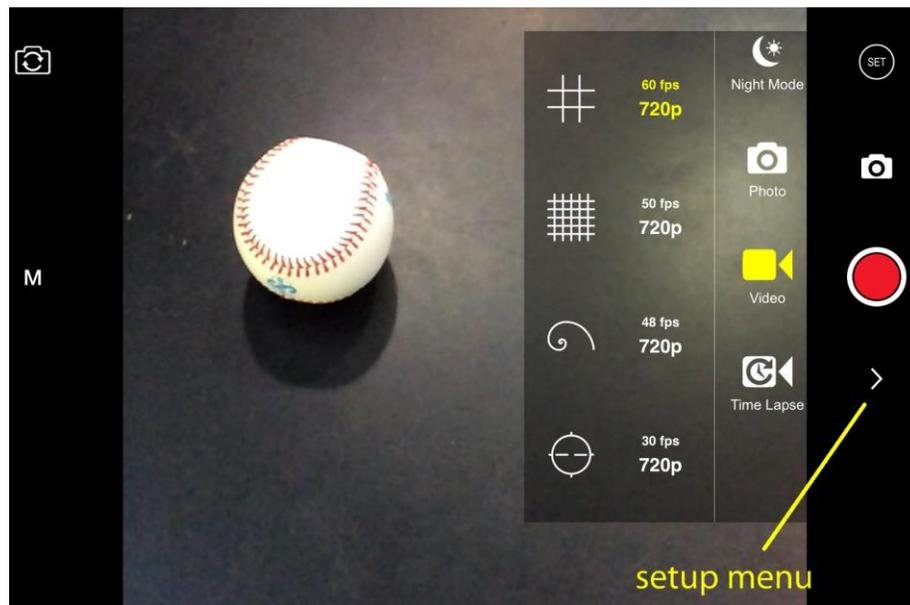
Make sure that the program is set to "video mode" (and not "camera mode") by selecting the "video" button. It should be highlighted yellow. The desired format is 60 fps or 120 fps - 720p; you can scroll vertically to find the appropriate format if it is not already selected.
