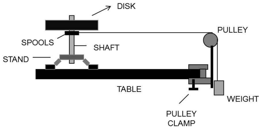
*Problem 3.2: Rotational dynamics apparatus. The string attached to the weight can be wrapped around either of two spools or to the perimeter of the disk.*
