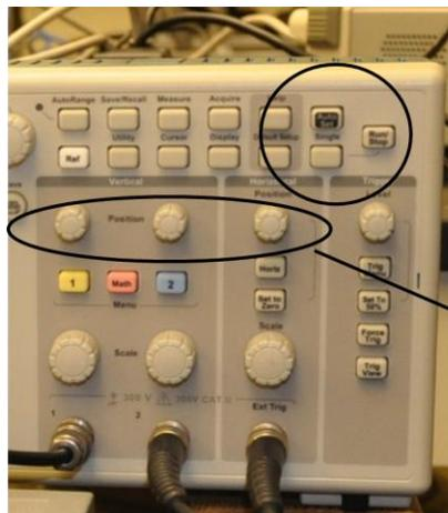
Hit the "Single" button to freeze the oscilloscope screen. Hit the "Run/Stop" button to resume normal operation
