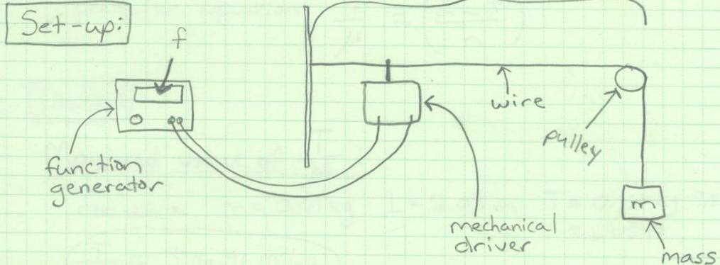
**Procedure:** Varied frequency ( $f$ ) to find  $n^{\text{th}}$  harmonic of wire for as many values of  $n$  as possible. Tension was provided by a hanging mass. The measured frequencies were used to determine the ratio  $\frac{T}{\mu}$ , where  $T$  = tension and  $\mu$  = mass density per length. This was then compared to the directly measured  $\frac{T}{\mu}$  of the wire. We did three trials.
