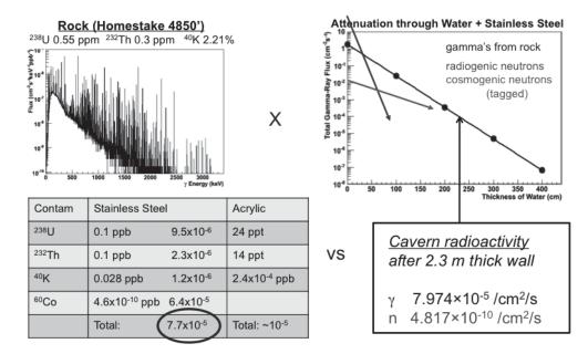
FIGURE 4. Optimization procedure to determine the minimum thickness of water between outside of stainless steel tank and inner tunnel lab. Geant4 Simulation using Homestake rock measurements as input (top left). Attenuation of gammas from the rock through a water shield of varying thickness (top right). Gamma levels due to contamination in the steel and acrylic itself (bottom left) compared to the level achieved after 2.3 m of water (bottom right).
