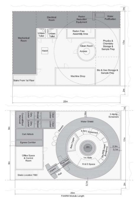
FIGURE 1. Floor plan for the DUSEL 4850' level Facility for Assay and Acquisition of Radiopure Materials, or FAARM.
