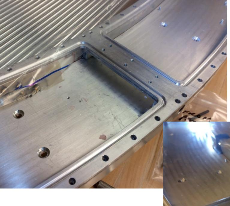
Aug 31-Sept 10: Removing excess epoxy from middle rib to install side panels.
