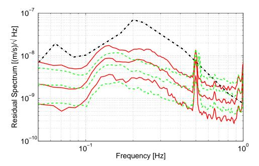
Figure 3. Plot comparing subtraction residuals over a month of data. The dashed curves are its 10th, 50th, and 90th percentiles using a filter that is updated once every day. The solid lines are the percentiles of residual noise using a filter updated once every week. The dash-dotted line in black represents the global new low-noise model [32].
