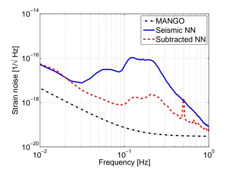
Figure 6. The MANGO GW detector target spectrum, as well as the NN estimate and its residual after suppression by the factor that was achieved with seismic data. There is about a factor of 50 subtraction across the microseism. A further order of magnitude subtraction will be required to achieve MANGO GW detector target sensitivity.
