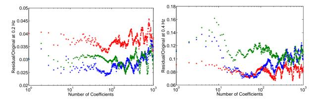
Figure 4. Residual noise evaluated over the three separate days as a function of filter order for the 800 ft target channel. The residuals shown in the plot on the left are evaluated at 0.2 Hz, whereas the residuals on the right are evaluated at 0.4 Hz.
