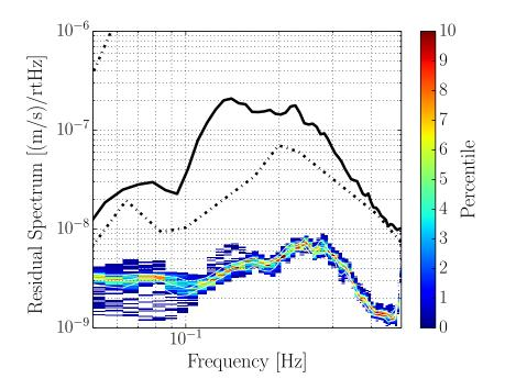
Figure 5. The plot shows the histogram of residual spectra for the 800 ft target channel achieved by each of the 1000 filter orders for the day represented by the blue markers in figure 4. The bottom, middle, and top white lines correspond to the 10th, 50th, and 90th percentiles respectively. The dash-dotted lines in black represent the global new low- and high-noise models [32]. The original spectra of the 800 ft channel is plotted in solid black.
