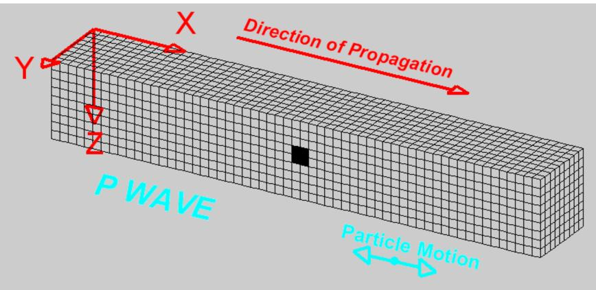
Deformation propagates. Particle motion consists of alternating compression and dilation. Particle motion is parallel to the direction of propagation (longitudinal). Material returns to its original shape after wave passes.
