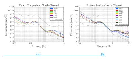
**Figure 2**: Median amplitude spectral densities for Homestake seismic stations. Numbered legend entries denote depth in feet, while numberless legend entries denote surface stations. Peterson low- and high-noise models are shown as dashed gray lines.
