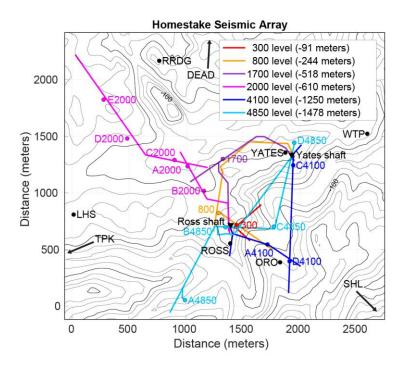
**Figure 1:** Homestake seismometer array layout. The lines of different colors depict the relevant drifts at various depths, along which we installed underground seismic stations. The black filled circles denote the surface stations (remote surface stations DEAD, SHL, and TPK were located approximately 2-3 km outside the depicted region). Also shown are the two shafts at the Homestake mine, known as the Yates and Ross shafts, denoted by black filled <u>reverse</u> triangles.
