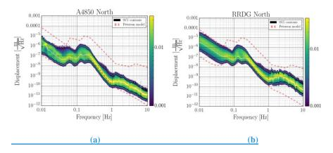
**Figure 3**: Histograms of amplitude spectral density in each frequency bin for an underground station at 4850 ft depth (aleft) and for a surface station (bright), calculated from 400-second data intervals over 1 year in each frequency bin. Median ASDs (solid
