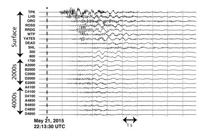
**Figure 5**: Vertical component seismograms from local surface mine. Seismograms are displayed at true amplitude and grouped by subarrays used throughout this paper.
