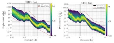
Figure 3: Histograms of amplitude spectral density in each frequency bin for a surface station (left) and for an underground station at 4850 ft depth (right). Median ASDs (solid white), 95% confidence intervals for each frequency bin (solid black), and the Peterson low- and high-noise models (dashed gray) are shown. See text for more details.
