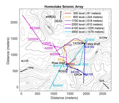
Figure 1: Homestake seismometer array layout. The lines of different colors depict the relevant drifts at various depths, along which we installed underground seismic stations. The black filled circles denote the surface stations (remote surface stations DEAD, SHL, and TPK were located outside the depicted region). Also shown are the two shafts at the Homestake mine, known as the Yates and Ross shafts, denoted by black filled triangles.
