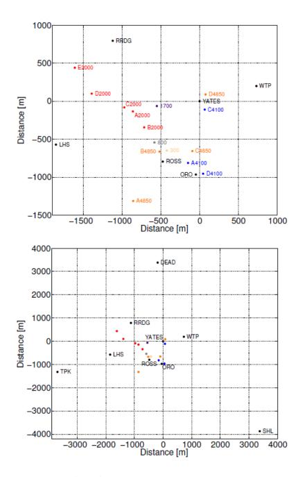
**Figure 1:** [PLACEHOLDER] Homestake array layout, relative to Yates shaft sation (at origin). A zoomed-in view with the underground stations labeled is shown on top (DEAD, SHL, and TPK not pictured). All stations are shown in the lower plot, but only the surface stations are labeled.
