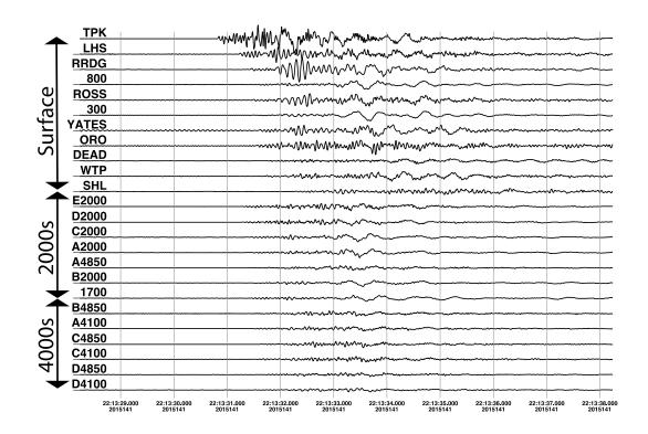
Figure LOCALBLAST. Vertical component seismograms from local surface mine. Seismograms are displayed at true amplitude an grouped by subarrays used throughout this paper. Records for each subarray are sorted by epicentral distance from the estimated source location (approximately 4 km west of TPK). Subarrays are ordered by increasing depth.
