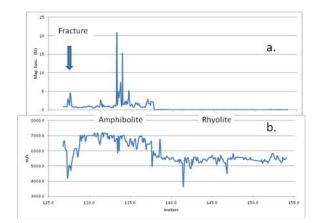
Fig. 4 a) Magnetic susceptibilities from a portion of Core C. b) Vp from the same portion of core. The rhyolite is characterized by lower velocities and magnetic susceptibilities. Healed fractures (meter marker 127 at arrow) in the amphibolite have lower seismic velocities and higher susceptibilities probably due to precipitation of pyrrhotite in the fractures.
