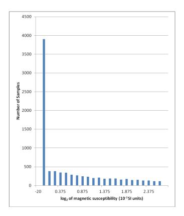
Fig. 5 Frequency distribution plot of magnetic susceptibility measurements of amphibolite samples. The results from a total of 8470 samples are shown in the plot although an additional 1158 samples plot to the left at higher susceptibilities but much lower frequency of occurrence.
