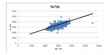
Fig. 3 Plot of Vp vs. Vs for all of the amphibolites measured in this study. The correlation between Vs and Vp is weak ( $R^2 = .6$ ) but yields a relationship of Vs = .4 Vp + 1060 m/s.
