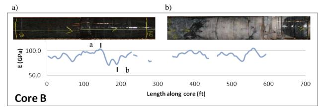
Fig. 6 Plot of E along the length of Core B for only the amphibolites showing the effect of changes in lithology. The gaps reflect the occurrence of rhyolites which are omitted from this plot. a) One foot (.3 m) core of amphibolite which represents the bulk of the rock mass shows a high value of E. b) Example of changes in lithology along the core length which may represent volumes of healed fractures.
