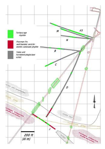
Fig. 1 Locations of drill holes on the 4850 of the Sanford Underground Research Facility (SURF). Cores from drill holes B, C, D, J, and a portion of N were used in this study that measured seismic velocities (Vp and Vs) and the magnetic susceptibility of the cored material. The units mapped during the Preliminary Design [10, 11] included the Yates amphibolite (grey), phyllite of the Poorman Formation (red), and Tertiary-age rhyolite(green).
