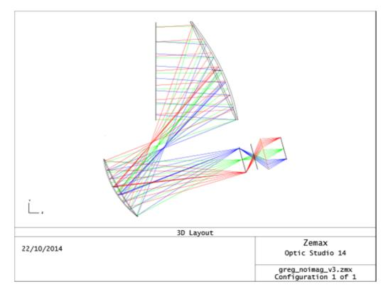
Figure 3: Gregorian design with re-imaging optics
