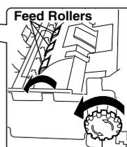
Feed Rollers should be cleaned by turning the Feed Rollers with the Paper Transport Knob.
