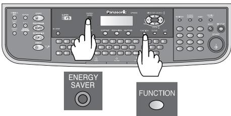
1. If the machine is in the "ENERGY SAVER (Shutdown Mode)", you may turn the Power Switch on the Left Side of the machine to the OFF position. If it is not in the "ENERGY SAVER (Shutdown Mode)", continue to step 2 below.
