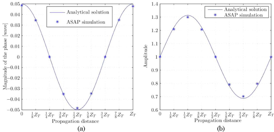
Fig. 7. (Color online) (a) Phase and (b) amplitude distribution at  $x = 0$  as a weak phase ripple propagates one Talbot distance. The results from the Fourier analysis were validated with numerical simulation using ASAP.
