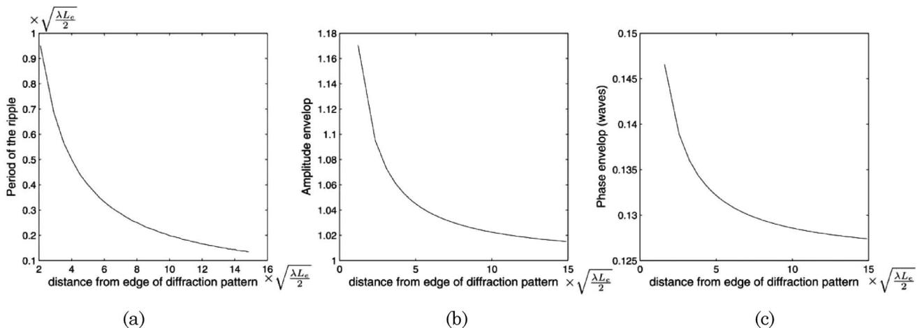
Fig. 6. (a) Period of the edge diffraction ripples, (b) the amplitude envelop, and (c) the phase envelop due to edge diffraction.
