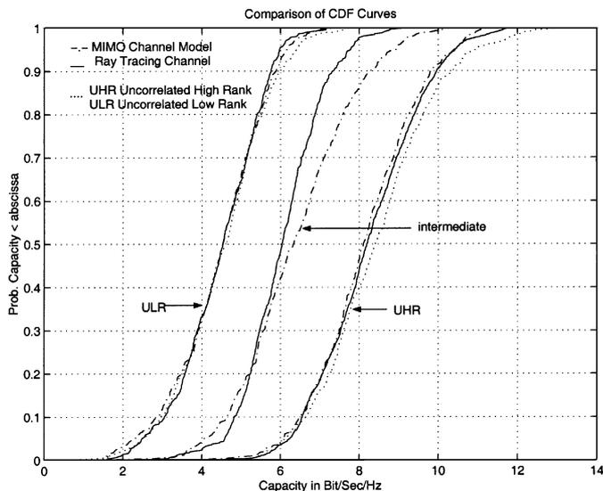
Fig. 7. Capacity cdf obtained with MIMO model for three sets of parameters. From left to right. Set 1:  $D_t = D_r = 30$  m,  $R = 1000$  km. Set 2:  $D_t = D_r = 50$  km,  $R = 50$  km. Set 3:  $D_t = D_r = 100$  m,  $R = 5$  km. The theoretical ULR and UHR models are plotted for comparison (dotted lines).
