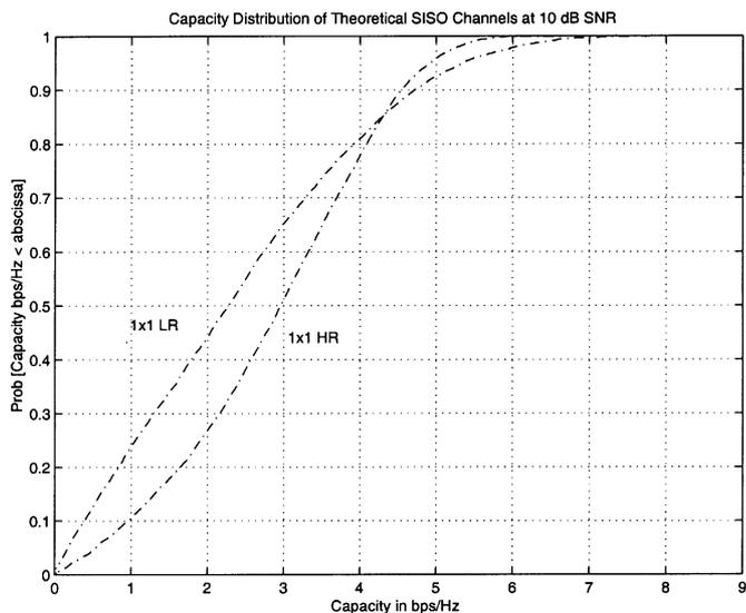
Fig. 2. Capacity curves for the 1x1 HR (Rayleigh) and 1x1 LR (double Rayleigh) channels. The double Rayleigh channel has worsened fading statistics.
