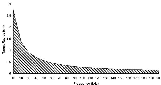
**Fig. 2** Range of frequencies and target radii over which the object becomes acoustically large (region above the hatched area) and reflects significant amounts of echo energy
