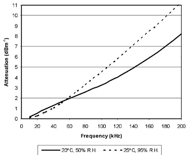
**Fig. 1** Atmospheric attenuation as a function of frequency for temperate regions of 20 °C and 50 per cent relative humidity and tropical regions of 25 °C and 95 per cent relative humidity
