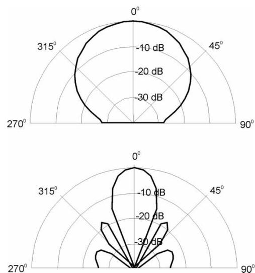
**Fig. 4** Beam pattern for a 10-mm diameter transducer producing a 40-kHz signal (top) and a 100-kHz signal (bottom)
