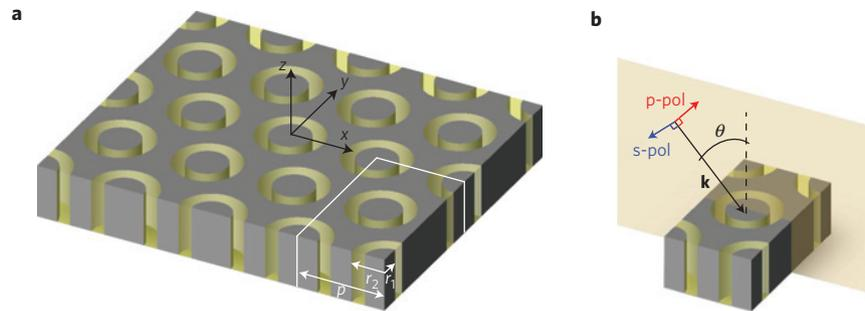
**Figure 1 | Negative-index metamaterial geometry.** **a**, Single-layer NIM slab consisting of a hexagonal array of subwavelength coaxial waveguide structures. The inner radius  $r_1$ , outer radius  $r_2$  and array pitch  $p$  are defined in the image. **b**, Unit cell of the periodic structure. The angle-of-incidence  $\theta$  is shown, as well as the in-plane (p-) and out-of-plane (s-) polarization directions associated with the incident wavevector  $\mathbf{k}$ .
