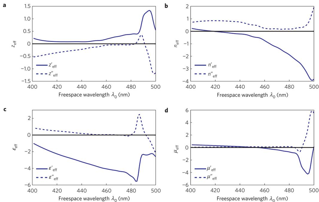
**Figure 4 | NIM effective parameters.** Effective parameters are calculated for a 100-nm-thick NIM slab excited at normal incidence over the 400–500 nm spectral range. **a–d**, The real (') and imaginary (") parts of the retrieved effective relative impedance  $z_{\text{eff}}$  (**a**), index  $n_{\text{eff}}$  (**b**), relative permittivity  $\epsilon_{\text{eff}}$  (**c**) and relative permeability  $\mu_{\text{eff}}$  (**d**).
